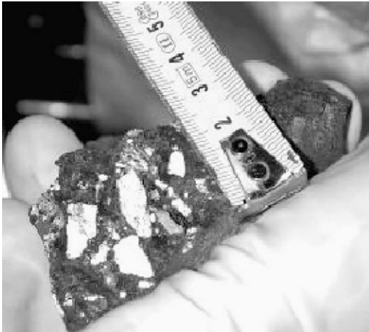
Fig. 13. Corium sample including unmelted siliceous aggregates.
