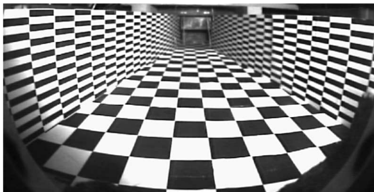
Fig. 3. Checkerboard used to calibrate the “fish-eye” camera before test VE-U1.
