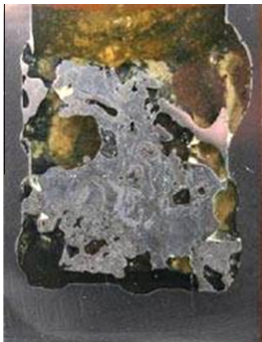
Fig. 7. Longitudinal section of a ZrC-coated crucible after the heating of 69.2 wt.% \text{UO}_2 + 8.5 wt.% \text{ZrO}_2 + 13.2 wt.% Zr + 9.1 wt.% steel mixture at 2320 °C.
