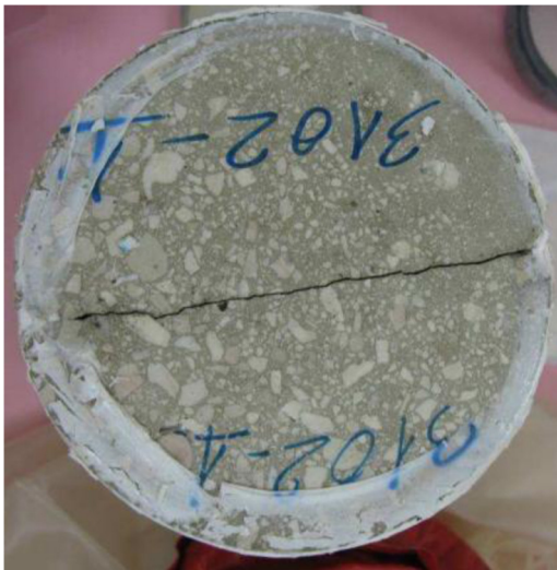
Fig. 6. Upstream face of the concrete sample after the test. The sample sealing is visible on its periphery.
