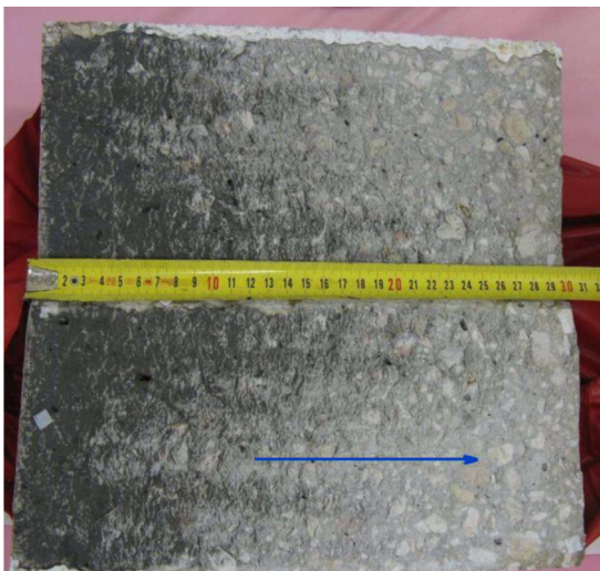
Fig. 7. Post-test view of the two sides of the concrete crack sample. The arrow indicates the direction of flow.
